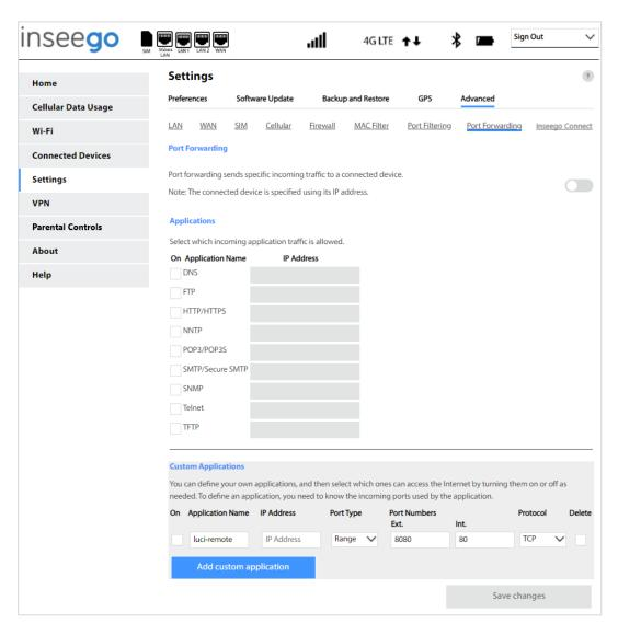
**NOTE:** When IP Passthrough is turned on, port forwarding capabilities are set through the connected host routing system. Settings on this page are not available. Go to **Advanced > LAN > IPPT** to turn IP Passthrough off.
