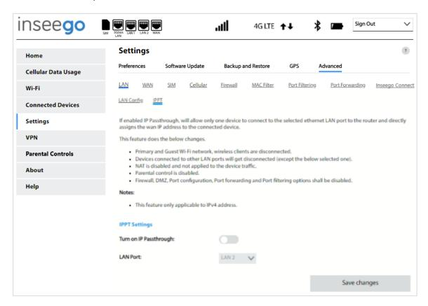
IP Passthrough (IPPT) enables the first device detected on the specified LAN port to obtain the IP address assigned by the mobile network. IPPT allows you to enable a one-to-one connection to a host routing system. **NOTE:** When IP Passthrough is on, only one device will have internet access. All other connected devices will be disconnected and lose internet access. The following capabilities are set through the host routing system and Web UI settings are not available:
