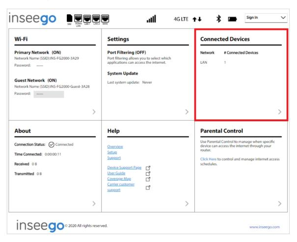
To manage connected devices, select > from the Home page Connected Devices panel (or select Connected Devices from the side menu).
