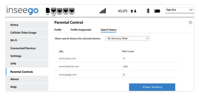
**NOTE:** You must first create a profile on the **Profile** tab and check the **URL Search History** check box. Then you must assign the profile to a device on the **Profile Assignment** tab.
