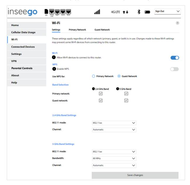
**NOTE:** When IP Passthrough is turned on, Wi-Fi networking capabilities are set through the connected host routing system. Settings on this page are not available. Go to **Advanced > LAN > IPPT** to turn IP Passthrough off.
