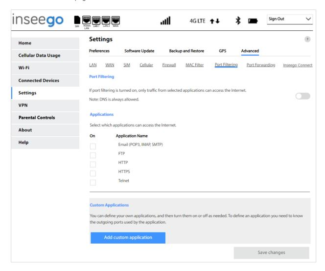
**NOTE:** When IP Passthrough is turned on, port filtering capabilities are set through the connected host routing system. Settings on this page are not available. Go to **Advanced > LAN > IPPT** to turn IP Passthrough off.
