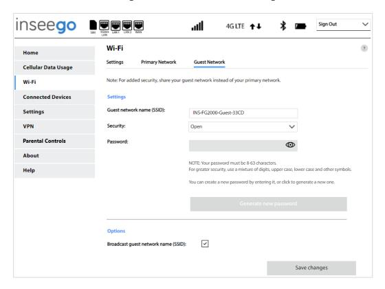
**NOTE:** When IP Passthrough is turned on, Wi-Fi networking capabilities are set through the connected host routing system. Settings on this page are not available. Go to **Advanced > LAN > IPPT** to turn IP Passthrough off.
