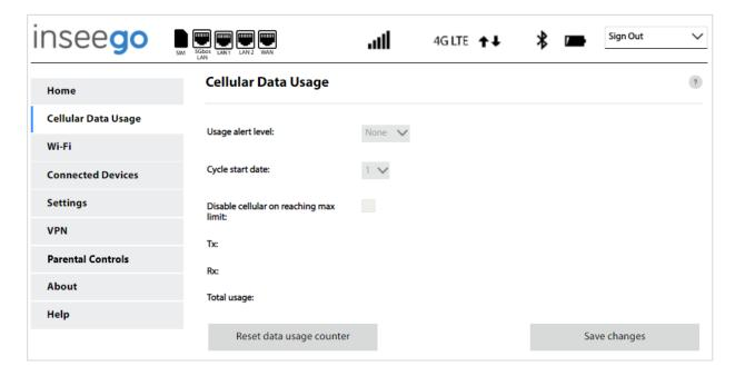
Usage alert level: Specify an alerting threshold for data usage (from 20 MB to 20 GB, or None).
