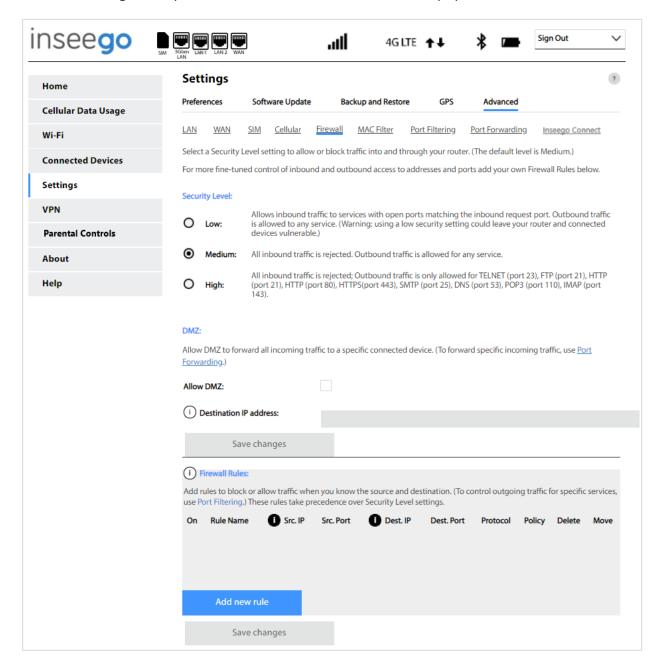
**NOTE:** When IP Passthrough is turned on, firewall capabilities are set through the connected host routing system. Settings on this page are not available. Go to **Advanced > LAN > IPPT** and turn IP Passthrough off.
