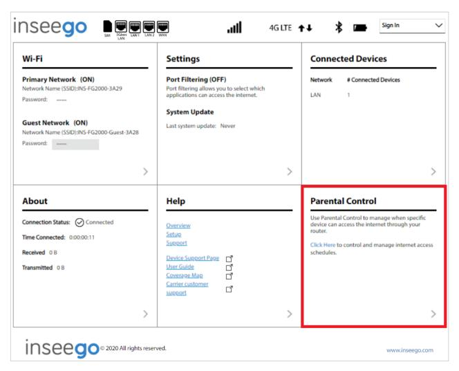
**NOTE:** When IP Passthrough is turned on, parental control capabilities are set through the connected host routing system. Parental control settings are not available on the Web UI. Go to **Advanced > LAN** > **IPPT** to turn IP Passthrough off.
