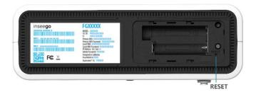
3. Press the SIM tool on the button for about five to six seconds, then your 5G Indoor CPE will restart.
