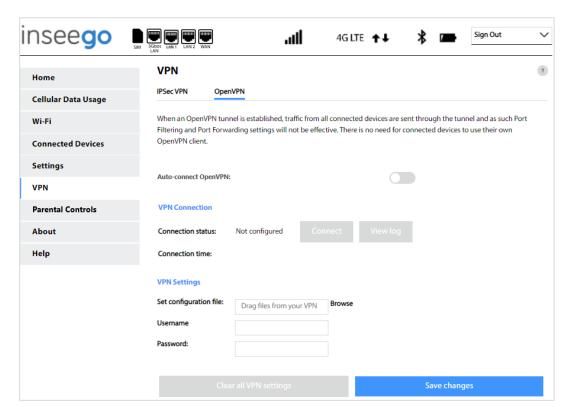
**NOTE:** When an OpenVPN connection is established, Port Filtering and Port Forwarding settings are not effective, as traffic from all connected devices goes through the OpenVPN tunnel.
