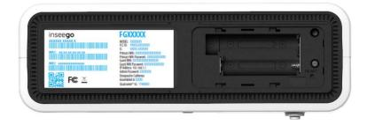
2. Insert three AA batteries following the diagrams on the router.
