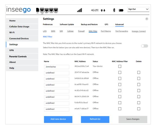
**NOTE:** The MAC filter has no effect on devices connected to the guest Wi-Fi network or devices connected via Ethernet.
